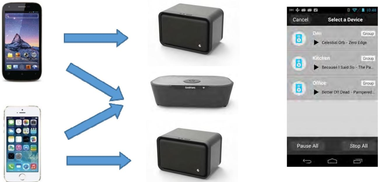
If several audio devices (AllPlay speakers, audio adaptors) are connected simultaneously on your home Wi-Fi network, you can play a song on speaker 1 and another song on the speaker 2 from any mobile device connected to the network.
