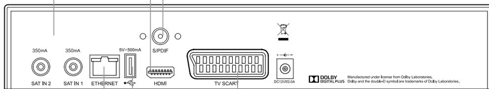
**ETHERNET** Connection to a network with broadband access (for IP TV Services such as BBC iPlayer).
