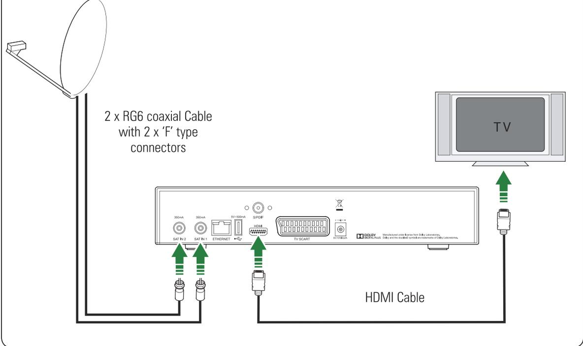
Connect two RG6 co-axial cables fitted with 'F' type connectors from your satellite dish to the 'SAT IN 1' and 'SAT IN 2' sockets on the back panel of your Digital TV Recorder.
