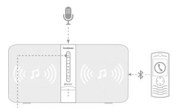
Press 'M' button until the indicator flashes blue quickly. Use your mobile phone to pair the Speaker.
