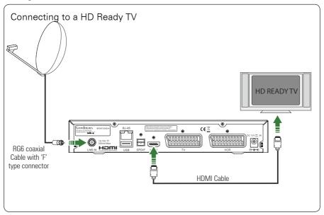
Connect a RG6 co-axial cable fitted with 'F' a type connector from your satellite dish to the 'LNB IN' socket on the back panel of your digital box.
