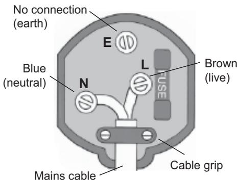
Make sure the outer sheath of the mains cable is securely held by the cable grip
