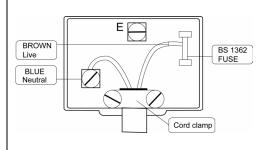
Blue.....Neutral Brown....Live The wires in this mains lead must be connected to the terminals in the plugs as follows: Blue Wire.....N or Black Brown Wire.....L or Red Only a 3 Amp fuse should be fitted in the plug or a 5 Amp fuse at the distribution board.
