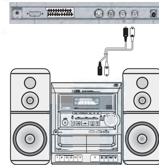
White audio left, red audio right RCA output connections on back of the TV to white audio left and red audio right RCA input connectors on audio system.
