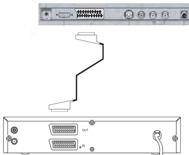
21 pin SCART connector from Socket 1 (TV In/ Out) to 21 pin SCART connector output on Digital set top box.
