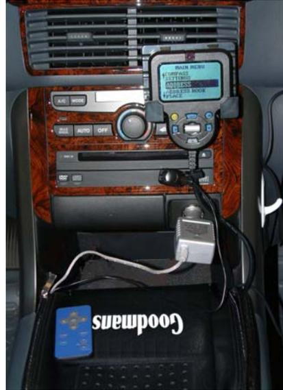
**Figure 2. Position Unit between Front Seats**
