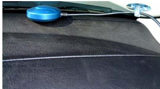
**Fig. 5 Position GPS Antenna under Windshield**
