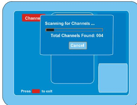
**Note:** The recorder will auto enter into TV mode after auto scanning all channels.
