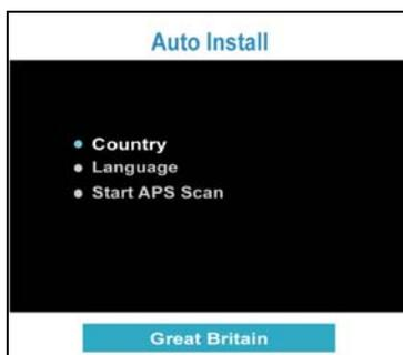
When you switch on the TV for the first time, the **Auto Install** menu will appear on the screen. (Make that a TV aerial is connected)
