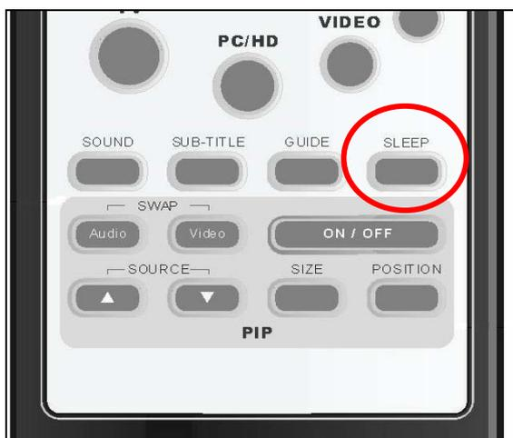
You can set the **Sleep Timer** to turn off the TV automatically. The timer can be set from 00 to 120 minutes.
