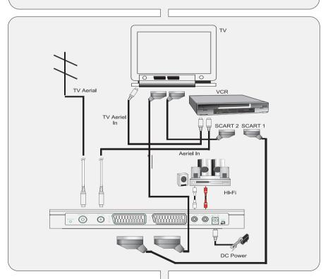
You can now record digital terrestrial programmes by selecting SCART 1 on the VCR. The VCR will also be able to record analogue television channels in the usual way. Both live and recorded digital terrestrial television programmes can be viewed on the TV by selecting the TV's AV input.GDB8 should be kept in TV viewing but not VCR viewing all the time in this connection.
