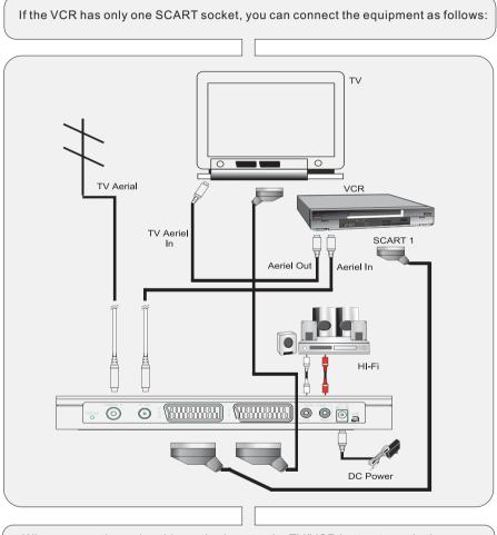
When connecting using this method, press the TV/VCR button to cycle the output from the TV SCART socket between DIGITAL TV output and the input from the VCR SCART socket.
