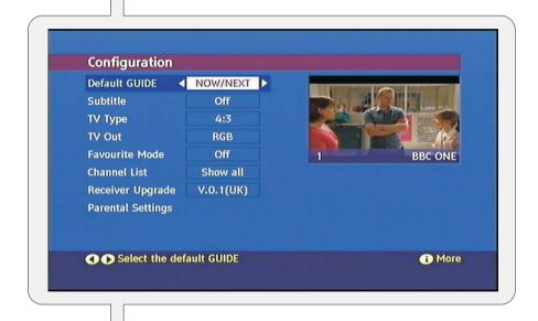
The various configuration functions are displayed in a list, along with quarterscreen image of the currently selected channel. You can select a function by highlighting the corresponding menu line with the UP or DOWN keys. There are eight configuration functions.
