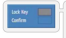
You must return to normal TV viewing by pressing the MENU key (three times) to activate the lock. Now any attempt to access the locked menus will display the PIN request window and the menus will only be displayed on entry of the correct PIN code.
