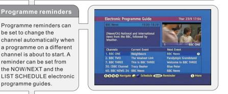
With the NOW/NEXT EPG screen showing, press RIGHT to display the next programme details in the text window and highlight the name of the next programme in the list of channels. Press SELECT when a programme you want to watch is highlighted and the reminder icon is displayed against that programme's name
