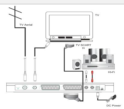
If you have a VCR or other equipment connected to your television, please connect the receiver as described here and refer to Appendix C later when satisfied that the receiver is functioning normally.
