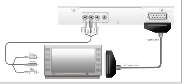
Connect the player's video (V), down mix audio left(L), right (R) output to the TV's video, audio left and right input.
