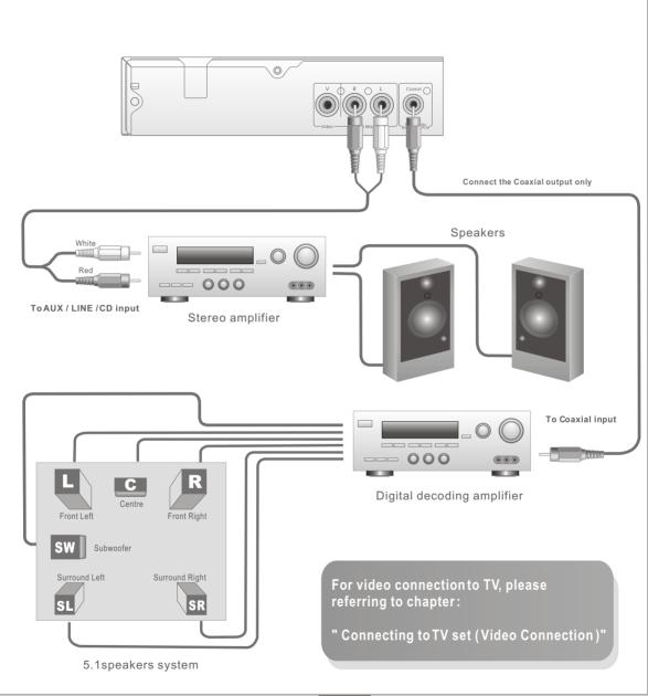
The player provide audio outputs for external stereo amplifier, or external digital amplifier (with Dolby Digital 5.1 decoding).
